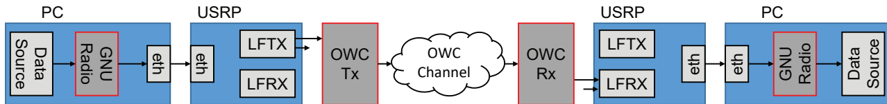
Figure 3. SDR-Based signal chain for IM/DD OWC with modular Tx/Rx hardware and parameterizable signal processing within the GNURadio toolkit using the gr-owc library.
