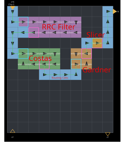
Figure 2. One BPSK receiver, 2 views. Left: the GNU Radio flowgraph the user draws, a Kyttar Source feeding an RRC matched filter, a complex Costas loop, a Gardner timing recovery, and a BPSK slicer, out to a Kyttar Sink. Right: the same design placed and routed on the 120-cell array. Each block becomes a coloured region of cells sized to the work it does, the RRC matched filter spanning 11 cells and the Costas loop 8, while the connections between blocks become routes across the grid (green). The blue cells carry data without computing on it. The graph the user drew is the layout on the silicon.
