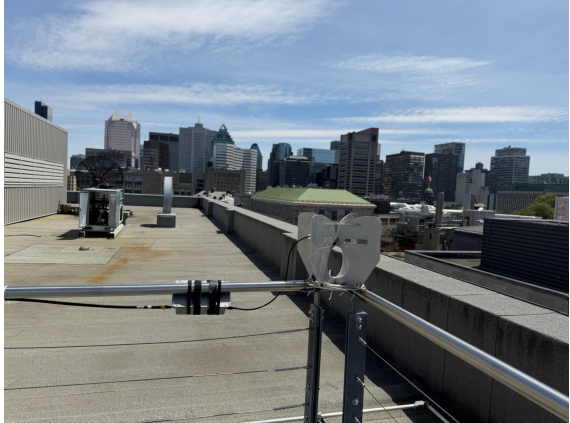
ublox-receiver Measured Beam 1575.420 MHz GALILEO (antenna height: 132 cm)
