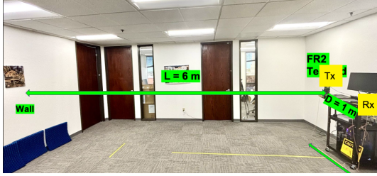
Figure 6. Indoor FR2 OTA empty-room baseline setup using one Sivers TX, one Sivers RX, the USRP X410, and OctoClock synchronization.
