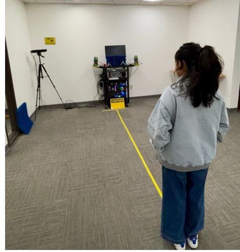
Figure 7. Indoor FR2 OTA sensing setup after introducing a static human target at approximately 3 m.
