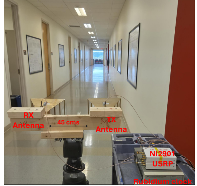
Figure 3. Bistatic testbed: NI USRP-2901 transmitter and two-channel sensing receiver sharing a rubidium reference, with TX and RX horn antennas on a 45 cm baseline aimed along the corridor.
